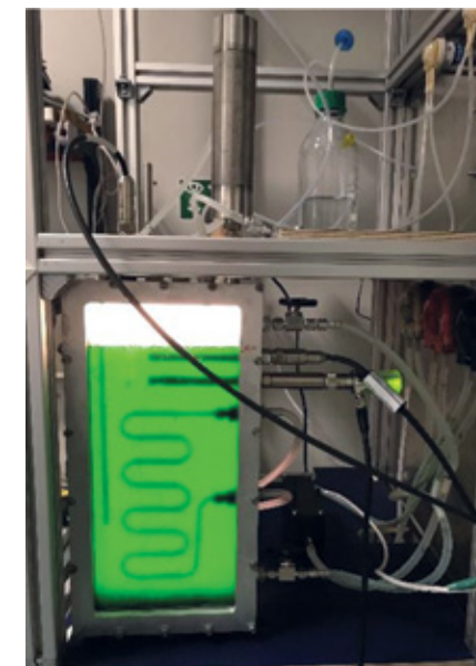
Figure 1: (Left) Configuration of the PBR. (Right) Course of OD 750 and OD 860 during the eight-day experiment with the improved configuration. The measurements at OD 750 are indicating a typical growth curve for cyanobacteria. Although the measurements OD 860 are less accurate, they have a similar progression to the measurements at OD 750 . The sensor setup was optimized using the Arc Wi Adapter (OD 860 sg), resulting in minimized noise and a smoother signal.
